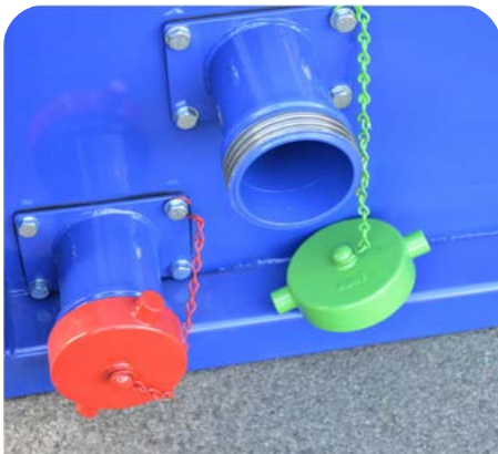
Top discharge outlet ( green ) Is used for water outlet.
