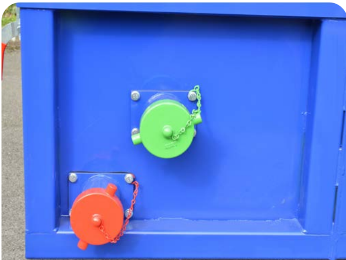
Bottom maintenance outlet ( red ) located either side of the filter head
