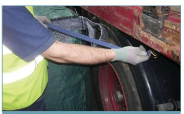
2. Fit claw hooks to vehicle rave and adjust strap and tension to ensure tight fit.
