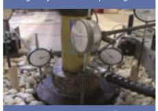
NTEC's compression and flow testing facility for load bearing surfaces.
