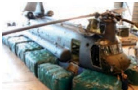
For safer working at height, Aviation soft landing bags can be linked and stacked around aircraft during maintenance.
