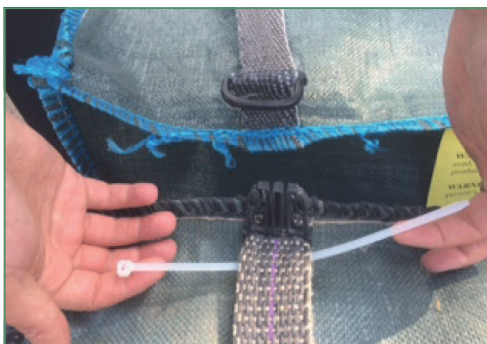
1. Place cable tie under one strap on either bag
