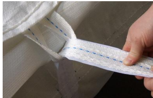
4) Secure lid of Wallet Bag using integral loops/straps.
